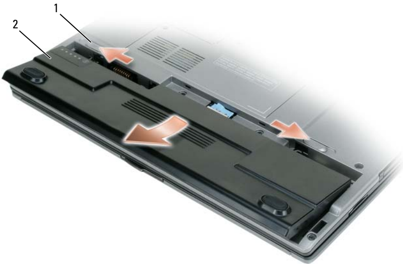
1 battery-bay release latch (2) battery
